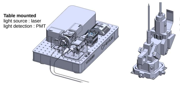
Head mounted optics and scanning mirrors
