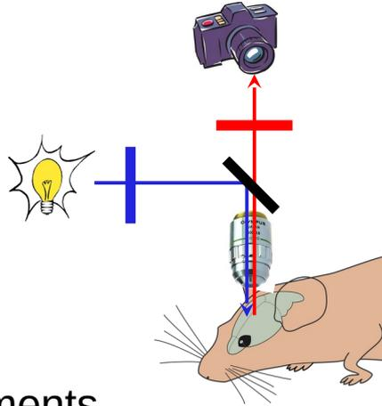
**1)** Minimize relative movements between animal to be imaged and the microscope
