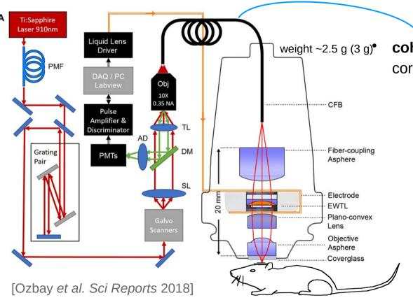
**coherent fiber bundle :** ~15,000 cores, core diameter ~2.9 μm, spacing ~4.5 μm
