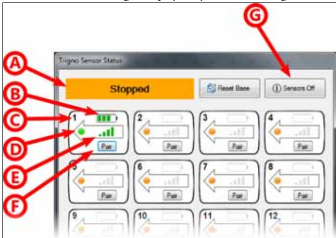
Figure 10. The Trigno Sensor Status Console offers real-time sensor feedback. A) data acquisition status, B) battery charge state, C) sensor number, D) sensor power, E) wireless signal strength, F) sensor pairing, G) off command.
