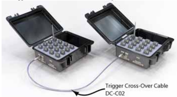
Figure 23. Installation of the Trigger Cross-Over cable to synchronize two base stations when used with EMGworks.
