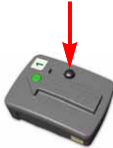
Figure 6. Turning the Trigno Sensor “ON”.
